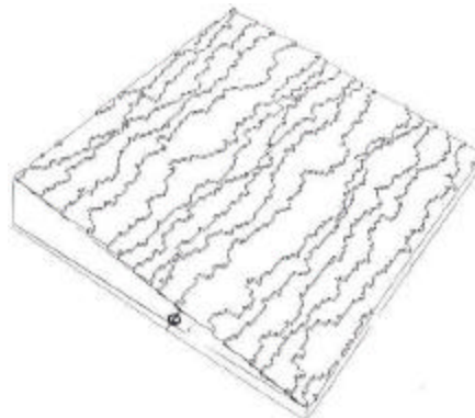
FIG. 3. Illustration of a stepped surface with meandering steps, specifically a Monte Carlo simulation of the terrace-step-kink model.
